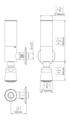
Installation: Exposed wall mounted Power supply: 9V battery **Operating pressure:** 0.5-8.0 bar (7-116 PSI) Water supply: Cold and premixed water Default water flow: 9 lpm / 2.38 gpm Water saving options with flow restrictor: • 7 lpm / 1.85 gpm
