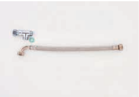
BELOW DECK TMV CONNECTION KIT Includes 1 x flexible hose 3/8", 1 x 90° brass arch, 1 x T-piece 3/8" Ref: 07291113
